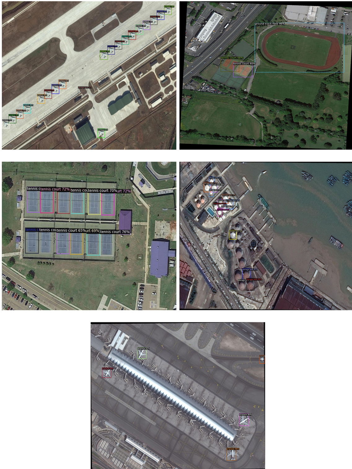
Fig. 4 Visualization of the objects detected by proposed framework using DOTA dataset. The figure also shows the confidence value and bounding box of each predicted object in the given image (best view zoom in)
